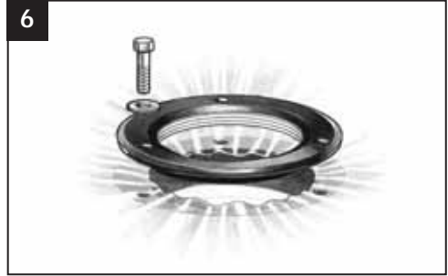
6. Where applicable, dress the membrane over the flange and into the sump of the body, ensuring that the membrane does not restrict the outlet; bolt the membrane clamping collar to the body – certain collars are reversible to increase height adjustability.
