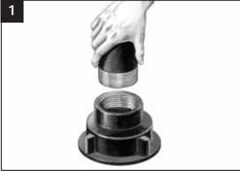
1. Where applicable, screw spigot adaptor into the body outlet using a suitable sealant to ensure the joint is watertight.
